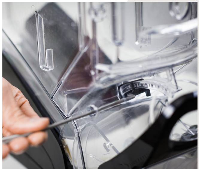
2. To achieve the greatest possible flow, push the small black device to the front of the ridge it sits on.
